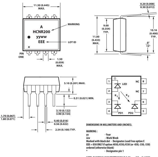
NOTE: FLOATING LEAD PROTRUSION IS 0.25 mm (10 mils) MAX.
