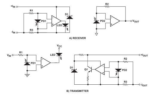
Figure 17: High-Speed Low-Cost Analog Isolator
