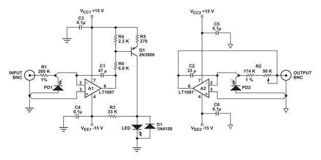
Figure 19: Bipolar Isolation Amplifier
