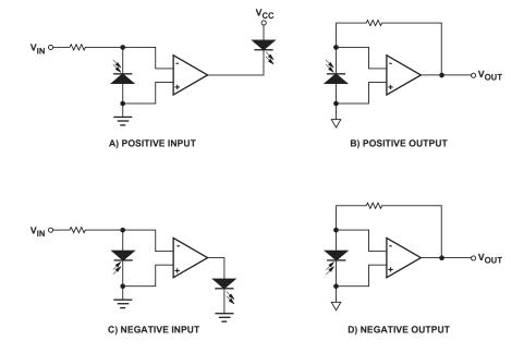
Figure 15: Bipolar Circuit Topologies
