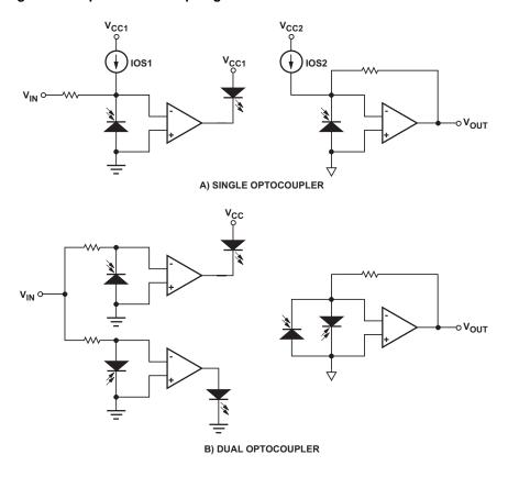
Figure 16: Loop-Powered 4 mA to 20 mA Current Loop Circuits
