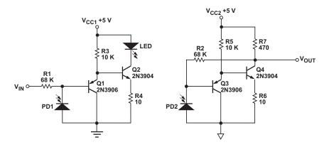
Figure 18: Precision Analog Isolation Amplifier
