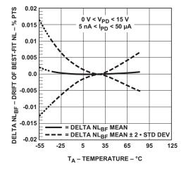
Figure 4: K3 Drift vs. Temperature
