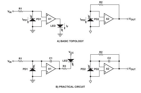
Figure 14: Unipolar Circuit Topologies
