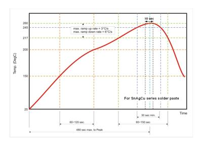
Fig 2. Infrared soldering profile
