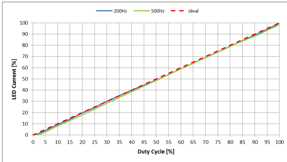
Figure 14. PWM Dimming Linearity
