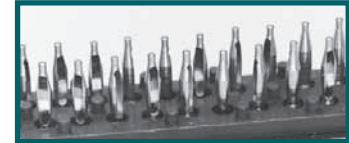
“Bi-Spring” Termination utilized on signal contacts
