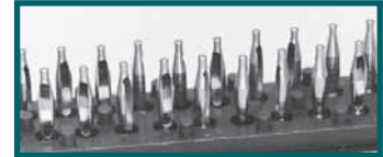
“Bi-Spring” Termination utilized on signal contacts
