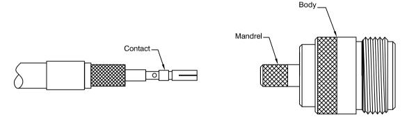
3) Insert the contact into the body and ensure that the contact captivates. Make sure the braid is on the outside of the mandrel. Slide the ferrule over the braid until the ferrule butts up against the body. Crimp the ferrule using the correct tool for the connector.
