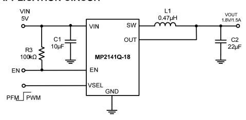
Figure 11: Typical Application Circuit NOTE: VIN < 3.3V may need more input capacitors.
