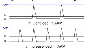
Figure 6: AAM Comparator Control Ton
