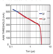
Figure 9: AAM Threshold Decreasing as Ton Increases
