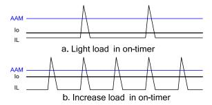
Figure 7: On-Timer Control Ton
