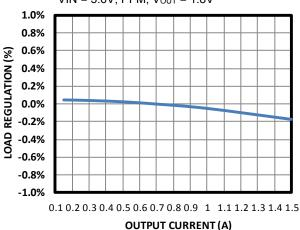
Load Regulation vs. Output Current
