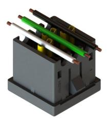
4 Use the cover to press the wire down into the IDC contacts. The cover must snap-in with the body.
