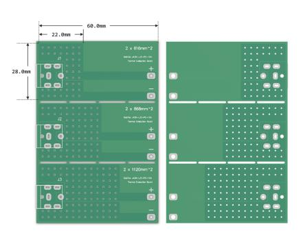
Above: GlobTek Thermal Evaluation Board for JACK-L-PC-10A-RA(R) and JACK-C-PC-10A-RA(R) Copper thickness: 2oz (0.071mm)
