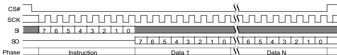
Figure 117. Password Read (PASSRD E7h) Command Sequence
