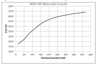
Figure 8: 6W CCT vs. Forward Current, T<sub>c</sub>=25°C
