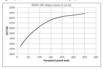
Figure 6: 4W CCT vs. Forward Current, T\_=25°C
