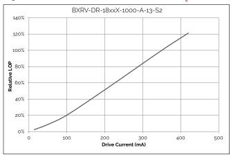
Figure 13: 12W Relative LOP vs. Drive Current,  $T_c$ =25°C
