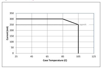
Figure 17: Derating Curve 6W, 12W
