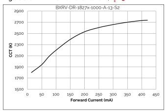
Figure 9: 12W CCT vs. Forward Current, T<sub>c</sub>=25°C
