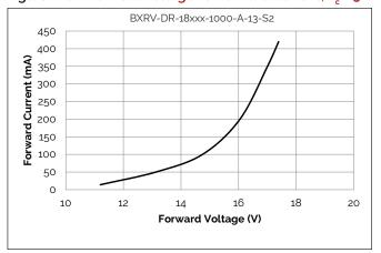
Figure 3: 12W Forward Voltage vs. Forward Current, T\_=25°C
