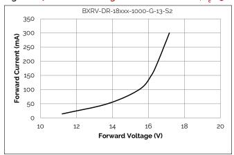
Figure 2: 6W Forward Voltage vs. Forward Current, T<sub>c</sub>=25°C
