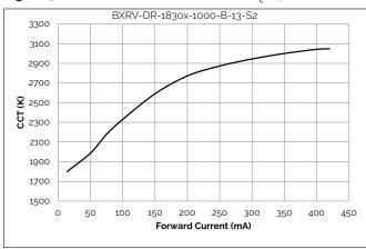
Figure 10: 12W CCT vs. Forward Current, T\_=25°C
