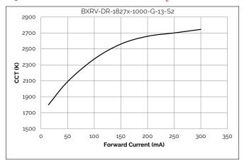
Figure 7: 6WCCT vs. Forward Current, T<sub>c</sub>=25°C
