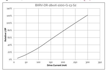
Figure 12: 6W Relative LOP vs. Drive Current, T<sub>c</sub>=25°C
