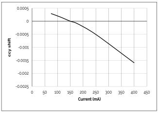
Figure 8: V8D Drive Current vs. ccx Shift
