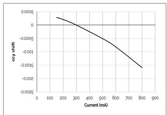
Figure 11: V8E Drive Current vs. ccy Shift
