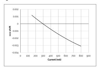
Figure 10: V8E Drive Current vs. ccx Shift
