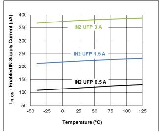
Figure 8. IN1 Current with UFP vs. Temperature
