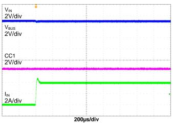
IN1 = IN2 = AUX = EN = 5V; CHG = CHG\_HI = 0V, CC1 = open, CC2 = Rd, OUT = open  $\rightarrow$  5  $\Omega$ Figure 13. Load Step
