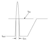
Figure 1. Output Short-Circuit Timing Diagram
