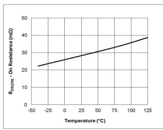
Figure 2. VBUS Current Limiting Switch On Resistance vs. Temperature
