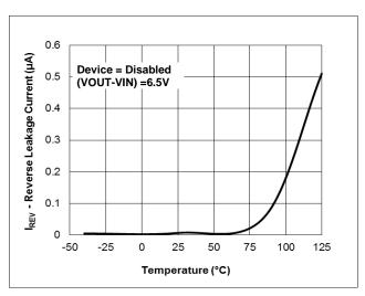
Figure 4. OUT Reverse Leakage Current vs. Temperature
