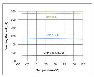
Figure 7. CC Sourcing Current to UFP vs. Temperature
