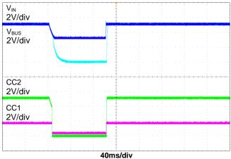
$$\begin{split} V_{\text{IN}} & 5V \rightarrow 3.5V \rightarrow 5V, \\ \text{IN1} & = \text{IN2} = \text{AUX} = \text{EN} = \text{CHG} = \text{CHG\_HI} = 5V, \\ & \text{CC1} = \text{Rd, CC2} = \text{Ra} \end{split}$$
