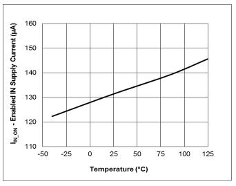
Figure 10. AUX Current with UFP vs. Temperature
