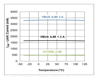
Figure 5. ILIM for VBUS and VCON vs. Temperature
