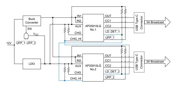
Figure 24. PPM and Power Wake Implemented
