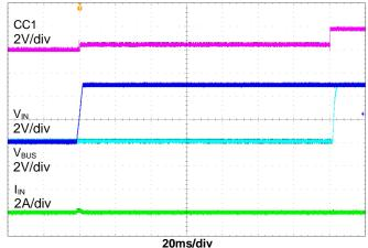
Basic start-up: IN1 = IN2 = AUX = EN = CHG = CHG\_HI = 5V, CC1 = Rd, CC2 = open Figure 11. Basic Start-Up
