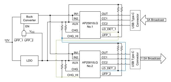
Figure 25. 3A USB Device Connected
