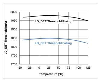
Figure 6. LD\_DET Threshold vs. Temperature
