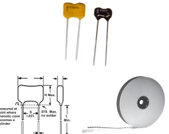
Type CDA15 is designed especially for auto-insertion and is the best value choice for tape and reel and ammo-pack feed systems. CDA15 is used in commercial and industrial applications requiring high stability, high Q and close capacitance tolerances. Type CDA15 is ideal for tuned circuits, delay lines and filter circuits.
