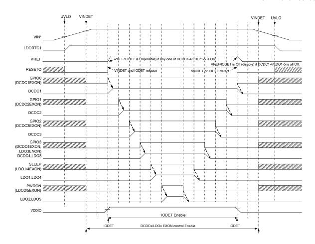
Fig. 8-1 Power On/Off function in Parts mode
