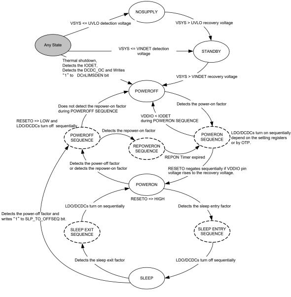
Fig. 6-1 Power Control State Machine Diagram
