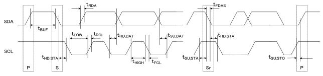
Fig. 10-3 I<sup>2</sup>C-Bus Interface Timing Chart
