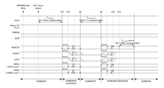
Fig. 6-6 Repower-on Sequence
