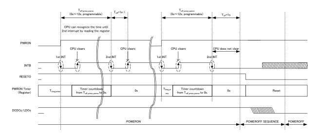
Fig. 6-11 PWRON Long Press Operation
