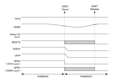
Fig. 6-9 Shutdown Sequence (IODET)
