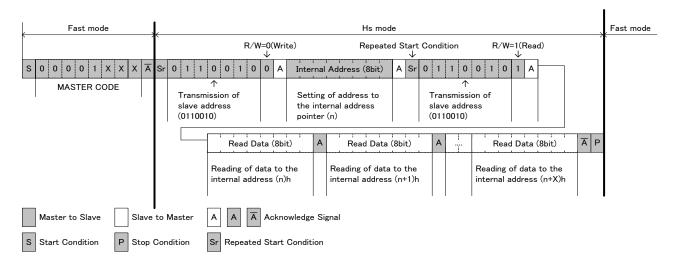
Fig. 10-4 I<sup>2</sup>C-Bus Data Transmission Read Format (Hs-mode)
