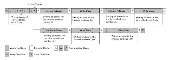
Fig. 10-2 I<sup>2</sup>C-Bus Data Transmission Write Format (Power I<sup>2</sup>C)
