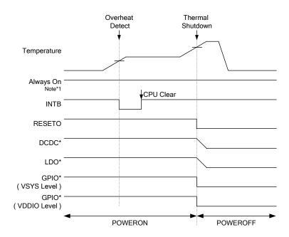
Fig. 6-8 Shutdown Sequence (Abnormal temperature)
