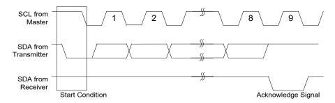
Fig. 10-4 I<sup>2</sup>C-Bus Data Transmission and Acknowledge
