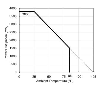
Power Dissipation vs. Ambient Temperature
