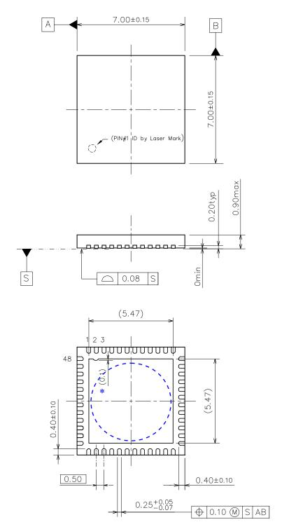
QFN0707-48-P25 Package Dimensions (Unit:mm)
