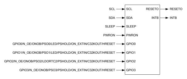
Fig. 8-1 The function of pins in Normal mode
