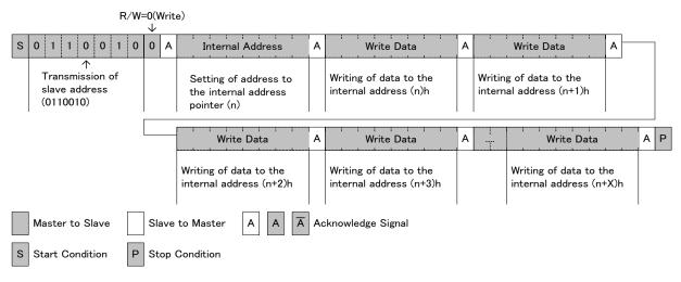
Fig. 10-1 I<sup>2</sup>C-Bus Data Transmission Write Format
