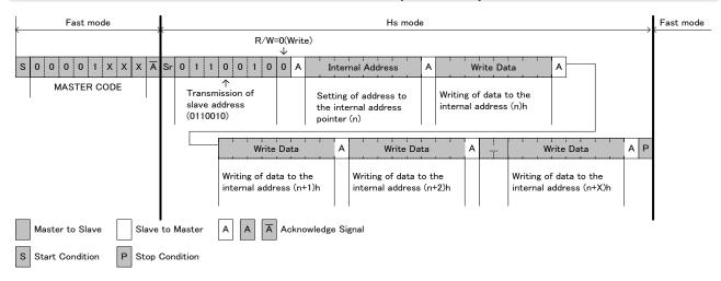
Fig. 10-5 I<sup>2</sup>C-Bus Data Transmission Write Format (Hs-mode)
