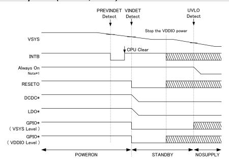
Fig. 6-7 Shutdown Sequence (VINDET, UVLO detection)
