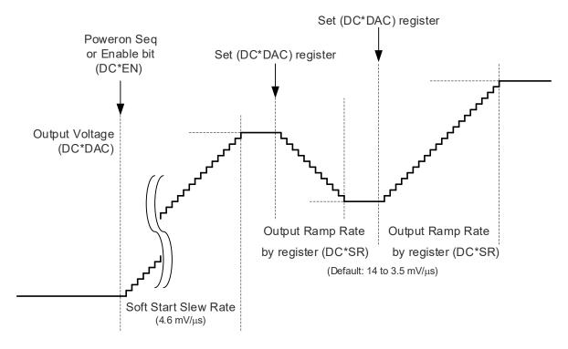
Fig. 7-1 Ramp up/down Control Timing Chart
