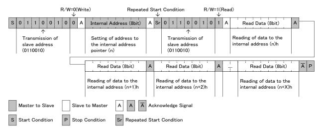
Fig. 10-5 I<sup>2</sup>C-Bus Data Transmission Read Format
