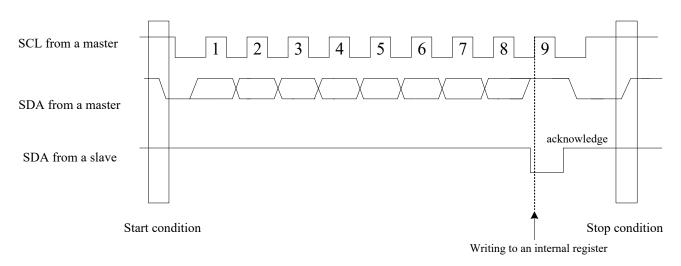
Fig. 10-3 I<sup>2</sup>C-Bus Internal Register Write-in Timing
