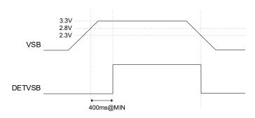
Fig. 6-12 Voltage Detection timing
