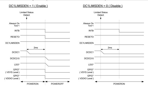
Fig. 6-10 Shutdown Sequence (DCDC1 current limit detection)
