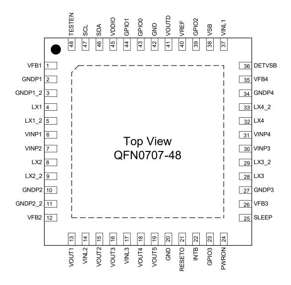
Fig. 5-1 Pin Configuration
