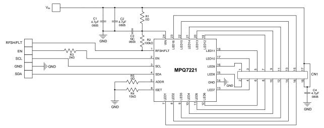
Figure 9: Typical Application Circuit (I<sub>LED</sub> = 80mA/Channel)
