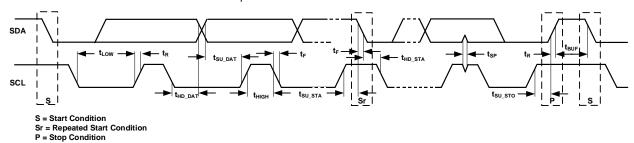
Figure 4: I<sup>2</sup>C-Compatible Interface Timing Diagram
