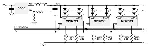
Figure 10: Typical System Application Circuit (2 LEDs in Series, I<sub>LED</sub> = 80mA/Channel)
