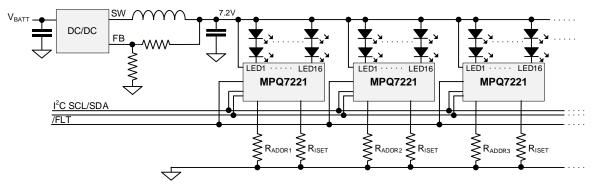
Figure 2: System Application Circuit with 2 LEDs in Series
