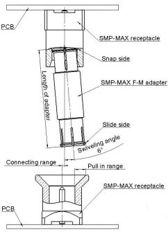
The connecting range represents the maximum misalignment during connection.
