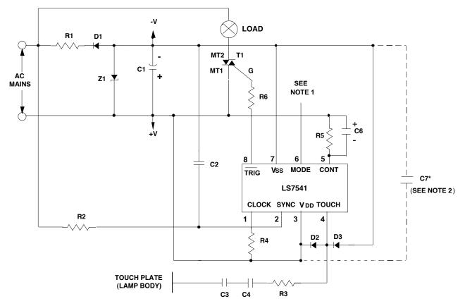
The Figure 5 Application Schematic functions identically to that shown in Figure 4 with one less component. Referencing Triac T1 to the +V power supply of the IC eliminates the need to AC couple the TRIAC pulse to the Triac Gate thereby eliminating component C5.
