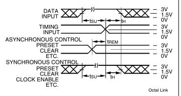
Set-up, Hold, and Release Times
