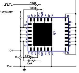
Fig. 24. Current sensing circuit
