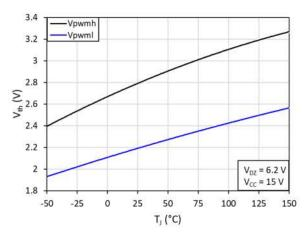
Fig. 7.  $V_{\text{PWMH}}$  and  $V_{\text{PWML}}$  vs. junction temperature(T\_J)
