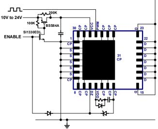
Fig. 22. Standby mode Vcc cut-off circuit
