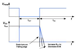
Fig. 23. Turn-on dV/dt slew rate control
