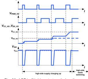
Fig. 20. ACF half-bridge start-up timing diagram
