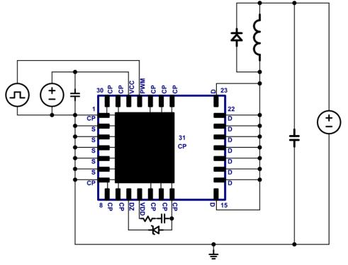
Fig. 1. Inductive switching circuit
