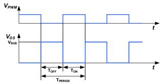
Fig. 21. Normal operating mode timing diagram
