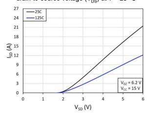
Fig. 5. Source-to-drain reverse conduction voltage
