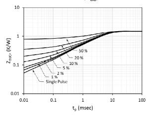
Fig. 17. Max. thermal transient impedance (Z  $_{thJC})$  vs. pulse width (t  $_{\rm P})$
