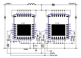
Fig. 25. Boost schematic using two parallel ICs
