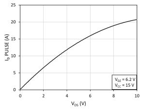
Fig. 4. Pulsed Drain current ( $I_D$  PULSE) vs. drain-to-source voltage ( $V_{DS}$ ) at T = 125 °C
