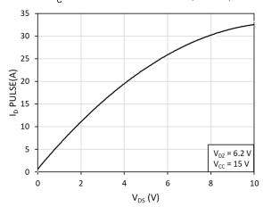
Fig. 3. Pulsed Drain current ( $I_D$  PULSE) vs. drain-to-source voltage ( $V_{DS}$ ) at T = 25 °C
