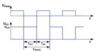
Fig. 21. Normal operating mode timing diagram
