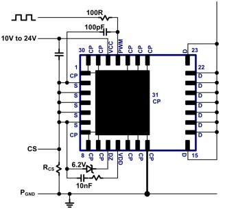
Fig. 24. Current sensing circuit
