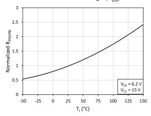
Fig. 8. Normalized on-resistance  $(R_{DS(ON)})$  vs. junction temperature  $(T_J)$
