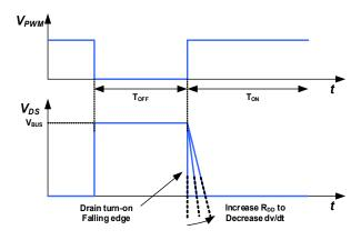
Fig. 23. Turn-on dV/dt slew rate control
