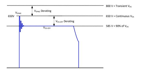
Fig. 28. QR flyback drain-to-source voltage stress diagram
