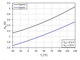
Fig. 7.  $V_{PWMH}$  and  $V_{PWML}$  vs. junction temperature  $(T_{.i})$
