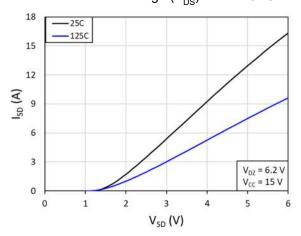
Fig. 5. Source-to-drain reverse conduction voltage
