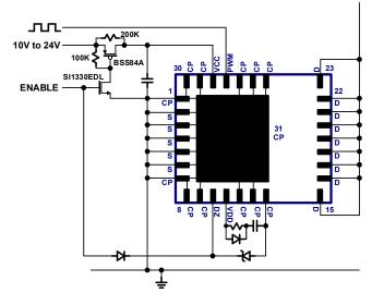
Fig. 22 Standby mode Vcc cut-off circuit
