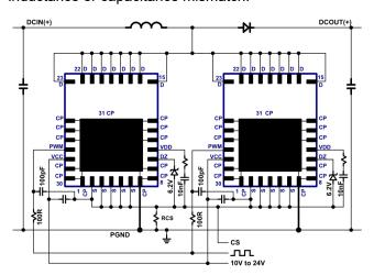
Fig. 25. Boost schematic using two parallel ICs
