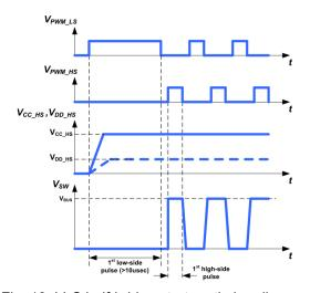
Fig. 19. LLC half-bridge start-up timing diagram
