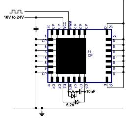
Fig. 18. Start-up circuit
