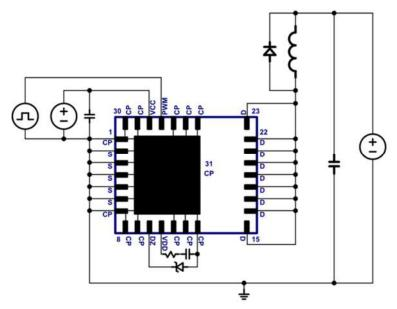
Fig. 1. Inductive switching circuit
