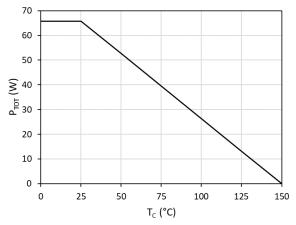
Fig. 16. Power dissipation ( $P_{TOT}$ ) vs. case temperature ( $T_{C}$ )
