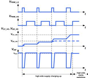
Fig. 20. ACF half-bridge start-up timing diagram
