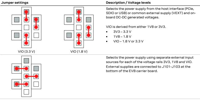
Table 7: Jumper settings (J1-J7) for selecting module input voltage
