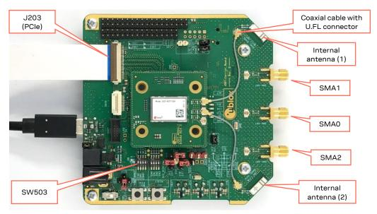
Figure 2: PCIe and USB connectors
