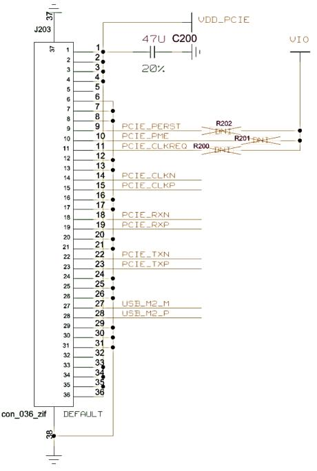
Figure 12: PCIe interface connector
