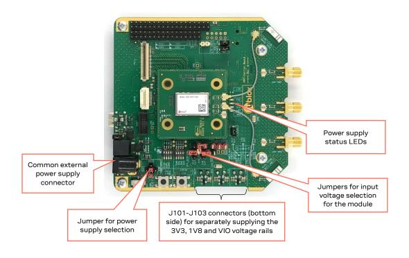
Figure 7: Overview of EVB power supply configuration
