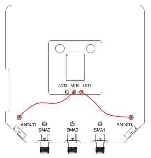
Figure 17: Default antenna configuration for EVK-JODY-W374
