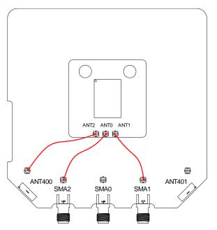
Figure 18: Default antenna configuration for EVK-JODY-W377
