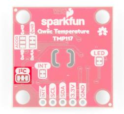
There is also a pull-up resistor on the  $\overline{INT}$  pin if you need to disable the it as well.
