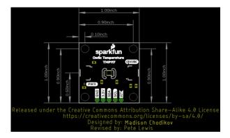
**Note:** For accurate readings, make sure to place the sensor horizontally and out of any airflow when mounting the sensor to an application.
