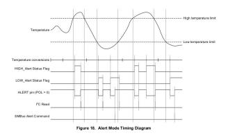
The example above shows what happens when we are in "alert mode." You'll notice that the flags and pin resets itself every time there is a read of the configuration register. If you modify the line that sets the alert function mode to "therm mode", the the flags behave slightly differently.
