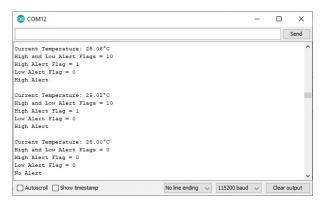
**Note:** If you look at *Figure 19 of the Therm Mode Timing Diagram* on page 16 of the datasheet, the serial output and the voltage of the pin matches what we expect from the TMP117!
