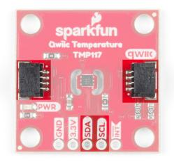
**Note:** For accurate readings, make sure to avoid heavy bypass traffic on the I<sup>2</sup>C bus and use the highest available communication speed. That is, try to not add too many I<sup>2</sup>C devices talking on the same bus or stretch your clock signal.
