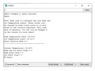
The current temperature reading at the time was 25.36°C. This is within the boundary of our temperature limits that we set so our alert flag is 0. You can adjust the limits as necessary but we made the temperature window narrow to easily test the functionality using the heat from our body. When we are outside the boundary limits, the alert flags will be set to 1 with their respective limits. As the temperature changes and is within our boundaries, the flag will be set back to 0.
