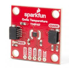
SparkFun High Precision Temperature Sensor - TMP117 (Qwiic) O SEN-15805
