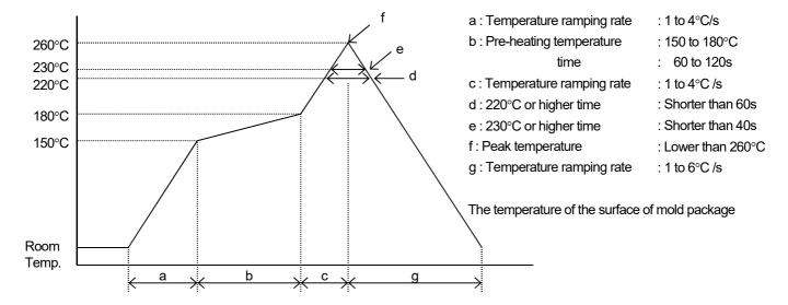
(NOTE1) Using reflow furnace with short wave infrared radiation heater such as halogen lamp Regarding temperature profile, please refer to those of reflow furnace.
