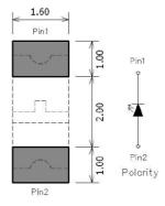
Figure 1. IN-S126BTNPD Solder Pattern
