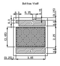
Unspecified tolerance:  $\pm 0.1$ mm Dimensions in parenthesis are shown for reference. 3.05
