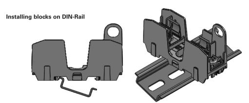
Place one edge of DIN-Rail in fuse block base, then rotate block down until it clicks into place.
