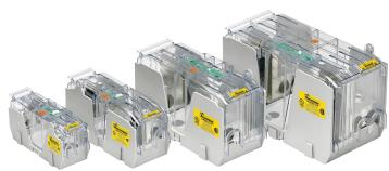
100 to 600 amp knifeblade fuse blocks are panel mount with multiple holes for installation flexibility and the modular design allows blocks to snap together for the desired number of poles. They accept optional snap-on covers for IP20 finger-safe protection and feature a lockout/tagout provision to improve electrical safety.
