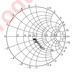
Condition:  $V_{CE} = 5 \text{ V}$ ,  $Z_{O} = 50 \Omega$ 100 to 2000 MHz (100 MHz Step)
