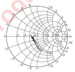
Condition:  $V_{CE} = 3 \text{ V}$ ,  $Z_{O} = 50 \Omega$ 100 to 2000 MHz (100 MHz Step)
