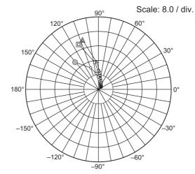
Condition:  $V_{CE} = 3 \text{ V}$ ,  $Z_{O} = 50 \Omega$ 100 to 2000 MHz (100 MHz Step)
