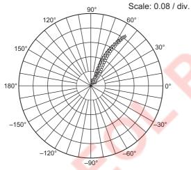
Condition: V<sub>CE</sub> = 3 V, Z<sub>O</sub> = 50  $\Omega$  100 to 2000 MHz (100 MHz Step)
