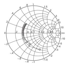
Condition:  $V_{CE} = 5 \text{ V}$ ,  $Z_{O} = 50 \Omega$ 100 to 2000 MHz (100 MHz Step)
