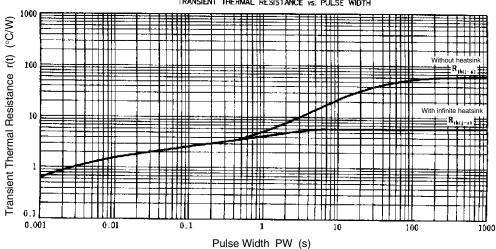
TRANSIENT THERMAL RESISTANCE vs. PULSE WIDTH
