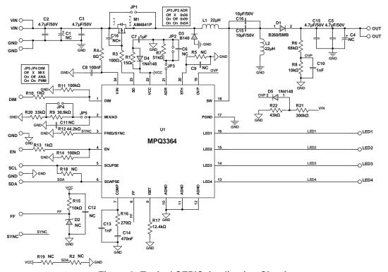
Figure 9: Typical SEPIC Application Circuit
