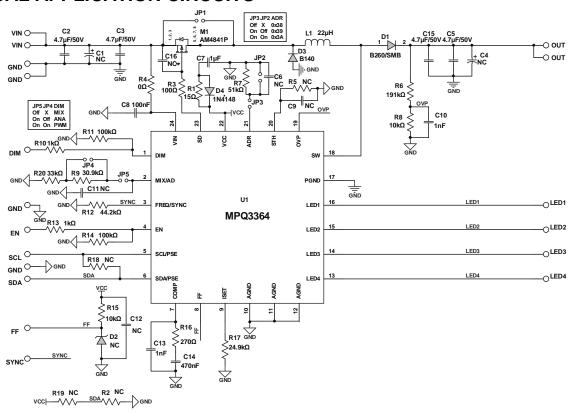
**Figure 8: Typical Boost Application Circuit**
