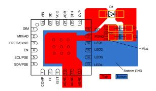
Figure 7: Recommended PCB Layout
