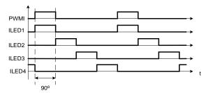
Figure 4: Phase Shift with 4 Channels
