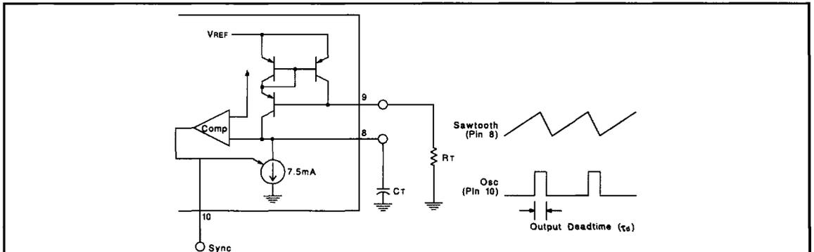
Output deadtime is determined by the external capacitor, CT, according to the formula:  $\tau_d (\mu s) = 145CT (\mu f) \left( \frac{I_D}{I_D - \frac{3.6}{RT (k\Omega)}} \right)$ .
