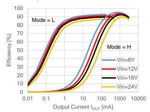
$V_{\text{OUT}} = 5.0 \text{ V}, f_{\text{OSC}} = 1000 \text{ kHz}$
