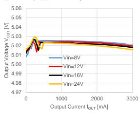
$V_{OUT} = 5.0 \text{ V}, f_{OSC} = 500 \text{ kHz}, Mode = H$
