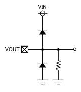
**Equivalent Circuit for VOUT Pin**
