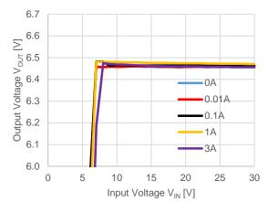
$V_{OUT} = 6.5 \text{ V}, \text{ fosc} = 500 \text{ kHz}, \text{ Mode} = \text{H}$
