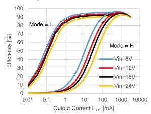
$V_{OUT} = 5.0 \text{ V}, \text{ fosc} = 500 \text{ kHz}$
