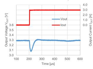
Vout = 3.3 V, V<sub>IN</sub> = 12 V, fosc = 500 kHz I<sub>OUT</sub> = 3 A  $\rightarrow$  0 A, Mode = H, Tf = 1 A/ $\mu$ s
