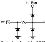
**Equivalent Circuit for RT Pin**
