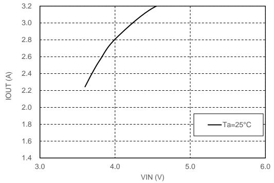
V<sub>OUT</sub> = 3.3 V / f<sub>OSC</sub> = 1MHz Setting R1276S Output Current vs Input Voltage
