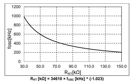
R1276S Oscillation Frequency vs. Oscillation Frequency Setting Resistor
