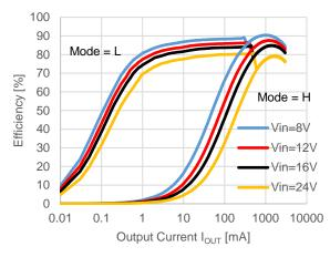
$V_{OUT} = 5.0 \text{ V}, \text{ fosc} = 250 \text{ kHz}$
