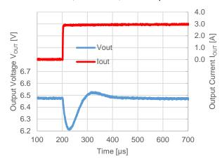
$V_{OUT} = 6.5 \text{ V}, V_{IN} = 12 \text{ V}, f_{OSC} = 500 \text{ kHz}$  $I_{OUT} = 3 \text{ A} \rightarrow 0 \text{ A}, Mode = H, Tf = 1 \text{ A/µs}$
