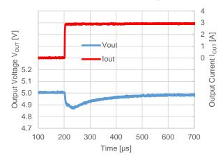
$V_{OUT} = 5.0 \text{ V}, V_{IN} = 12 \text{ V}, f_{OSC} = 500 \text{ kHz}$  $I_{OUT} = 3 \text{ A} \rightarrow 0 \text{ A}, Mode = L, Tf = 1 \text{ A/µs}$
