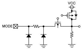
**Equivalent Circuit for MODE Pin**
