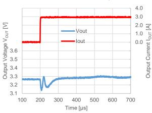
$V_{OUT} = 3.3V$ ,  $V_{IN} = 12V$ ,  $f_{OSC} = 500kHz$  $I_{OUT} = 3 A \rightarrow 0 A$ , Mode = L,  $Tf = 1 A/\mu s$
