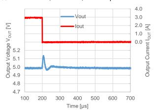
$V_{OUT} = 6.5 \text{ V}$ ,  $V_{IN} = 12 \text{ V}$ ,  $f_{OSC} = 500 \text{ kHz}$  $I_{OUT} = 0.1 \text{ A} \rightarrow 1 \text{ A}$ , Mode = L, Tr = 1 A/µs
