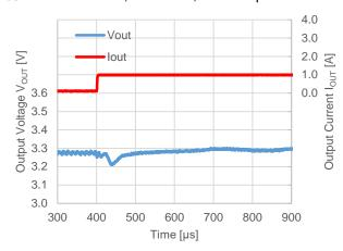
$V_{OUT} = 3.3 \text{ V}, V_{IN} = 12 \text{ V}, f_{OSC} = 500 \text{ kHz}$  $I_{OUT} = 1 \text{ A} \rightarrow 0.1 \text{ A}, Mode = L, Tf = 1 \text{ A/µs}$
