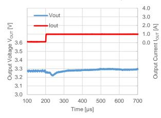
$V_{OUT} = 3.3 \text{ V}, V_{IN} = 12 \text{ V}, f_{OSC} = 500 \text{ kHz}$   $I_{OUT} = 1 \text{ A} \rightarrow 0.1 \text{ A}, Mode = H, Tf = 1 \text{ A/}\mu\text{s}$
