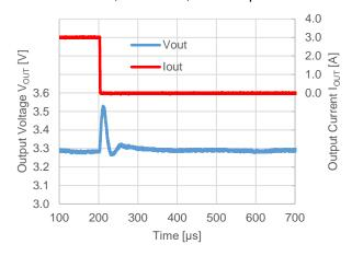
$V_{OUT} = 5.0 \text{ V}, V_{IN} = 12 \text{ V}, f_{OSC} = 500 \text{ kHz}$  $I_{OUT} = 0.1 \text{ A} \rightarrow 1 \text{ A}, Mode = L, Tr = 1 \text{ A/µs}$
