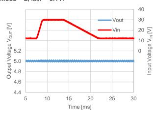
$fosc = 250 \text{ kHz}, V_{\text{IN}} = 12 \text{ V} \leftrightarrow 30 \text{ V}$   $Mode = H, I_{\text{OUT}} = 0.1 \text{ A}$
