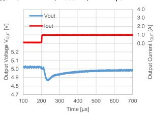
$V_{OUT} = 5.0 \text{ V}, V_{IN} = 12 \text{ V}, f_{OSC} = 500 \text{ kHz}$  $I_{OUT} = 1 \text{ A} \rightarrow 0.1 \text{ A}, Mode = L, Tf = 1 \text{ A/µs}$
