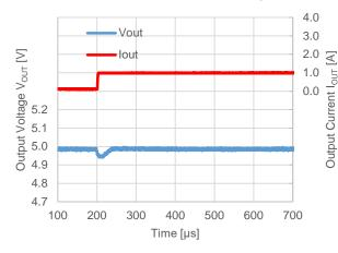
$V_{OUT} = 5.0 \text{ V}, V_{IN} = 12 \text{ V}, f_{OSC} = 500 \text{ kHz}$  $I_{OUT} = 1 \text{ A} \rightarrow 0.1 \text{ A}, Mode = H, Tf = 1 \text{ A/µs}$
