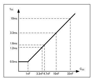
$$\begin{split} &C_{SS}\left[nF\right] = (t_{SS} - t_{VO\_S}) \: / \: 0.64 \times 2.0 \\ &t_{SS} : Soft\text{-start time (ms)} \\ &t_{VO\_S} : \text{Time period from } \\ &CE = \text{"High" to VOUT's rising} \\ &(\text{Typ. 0.160 ms}) \end{split}$$
