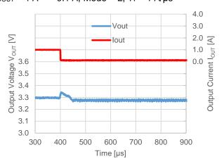
$V_{OUT} = 3.3 \text{ V}, V_{IN} = 12 \text{ V}, f_{OSC} = 500 \text{ kHz}$  $I_{OUT} = 0 \text{ A} \rightarrow 3 \text{ A}, \text{ Mode} = \text{L}, \text{Tr} = 1 \text{ A/µs}$
