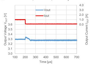
$V_{OUT} = 3.3 \text{ V}, V_{IN} = 12 \text{ V}, fosc = 500 \text{ kHz}$  $I_{OUT} = 0 \text{ A} \rightarrow 3 \text{ A}, Mode = H, Tr = 1 \text{ A/µs}$
