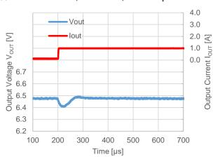
$V_{OUT} = 6.5 \text{ V}, V_{IN} = 12 \text{ V}, f_{OSC} = 500 \text{ kHz}$  $I_{OUT} = 1 \text{ A} \rightarrow 0.1 \text{ A}, Mode = H, Tf = 1 \text{ A/}\mu\text{s}$
