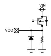
**Equivalent Circuit for VCC Pin**
