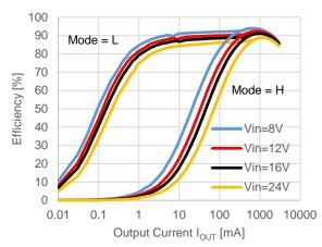
$$V_{OUT} = 3.3 \text{ V}, \text{ fosc} = 500 \text{ kHz}$$
