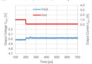
$V_{OUT} = 5.0 \text{ V}, V_{IN} = 12 \text{ V}, f_{OSC} = 500 \text{ kHz}$  $I_{OUT} = 0 \text{ A} \rightarrow 3 \text{ A}, Mode = L, Tr = 1 \text{ A/µs}$
