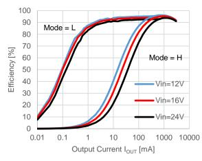
$V_{OUT} = 6.5 \text{ V}, \text{ fosc} = 500 \text{ kHz}$
