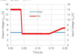
$f_{OSC} = 250 \text{ kHz}$ Mode = L,  $I_{OUT} = 0.1 \text{ A}$
