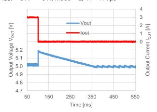
$V_{OUT} = 5.0 \text{ V}, V_{IN} = 12 \text{ V}, f_{OSC} = 500 \text{ kHz}$  $I_{OUT} = 0.1 \text{ A} \rightarrow 1 \text{ A}, Mode = H, Tr = 1 \text{ A/}\mu\text{s}$
