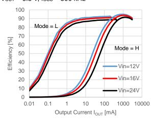
$V_{OUT} = 6.5 \text{ V}, f_{OSC} = 1000 \text{ kHz}$
