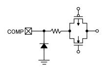
**Equivalent Circuit for COMP Pin**
