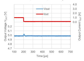
$V_{OUT} = 5.0 \text{ V}, V_{IN} = 12 \text{ V}, fosc = 500 \text{ kHz}$  $I_{OUT} = 0 \text{ A} \rightarrow 3 \text{ A}, Mode = H, Tr = 1 \text{ A/µs}$
