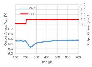
$V_{OUT} = 6.5 \text{ V}, V_{IN} = 12 \text{ V}, f_{OSC} = 500 \text{ kHz}$  $I_{OUT} = 1 \text{ A} \rightarrow 0.1 \text{ A}, Mode = L, Tf = 1 \text{ A/µs}$
