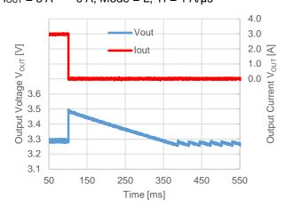
$V_{OUT} = 3.3 \text{ V}, V_{IN} = 12 \text{ V}, f_{OSC} = 500 \text{ kHz}$  $I_{OUT} = 0.1 \text{ A} \rightarrow 1 \text{ A}, Mode = L, Tr = 1 \text{ A/µs}$
