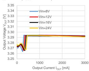
$V_{OUT} = 3.3 \text{ V}, \text{ fosc} = 500 \text{ kHz}, \text{ Mode} = \text{H}$
