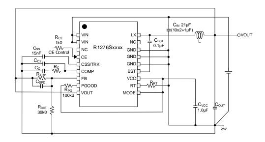
**Test Circuit for Typical Characteristics**
