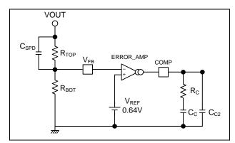
**Connection Example for External Phase Compensation Circuit**
