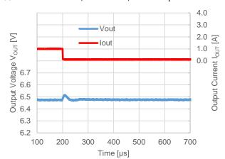
$V_{OUT} = 6.5 \text{ V}, V_{IN} = 12 \text{ V}, f_{OSC} = 500 \text{ kHz}$  $I_{OUT} = 0 \text{ A} \rightarrow 3 \text{ A}, Mode = H, Tr = 1 \text{ A/}\mu\text{s}$
