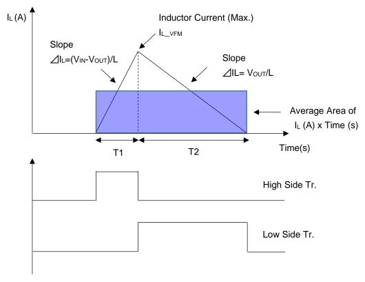
**Inductor Current Waveform at VFM Mode**
