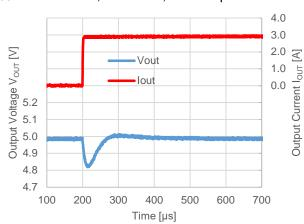
$V_{OUT} = 5.0 \text{ V}, V_{IN} = 12 \text{ V}, f_{OSC} = 500 \text{ kHz}$  $I_{OUT} = 3 \text{ A} \rightarrow 0 \text{ A}, Mode = H, Tf = 1 \text{ A/}\mu\text{s}$
