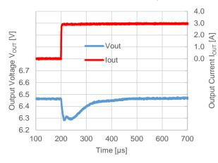
$V_{OUT} = 6.5 \text{ V}$ ,  $V_{IN} = 12 \text{ V}$ ,  $f_{OSC} = 500 \text{ kHz}$  $I_{OUT} = 3 \text{ A} \rightarrow 0 \text{ A}$ , Mode = L,  $T_{I} = 1 \text{ A/µs}$
