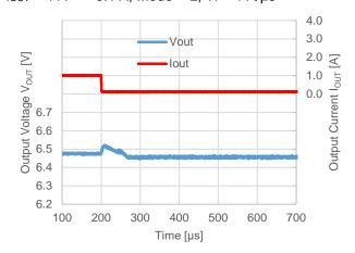
$V_{OUT} = 6.5 \text{ V}, V_{IN} = 12 \text{ V}, f_{OSC} = 500 \text{ kHz}$  $I_{OUT} = 0 \text{ A} \rightarrow 3 \text{ A}, Mode = L, Tr = 1 \text{ A/µs}$
