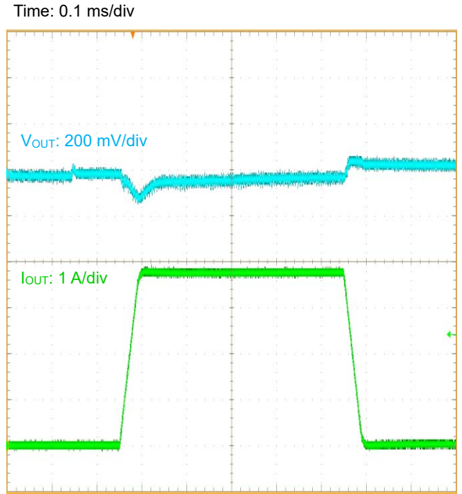
Figure 49. Load Transient Response ( V_{IN} = 36\text{ V} , I_{OUT} = 0\text{ A} - 3.75\text{ A} )
