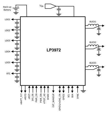
Figure 1. Simplified Application Circuit
