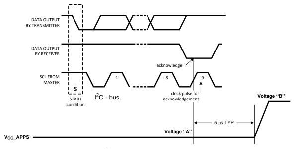
Figure 23. I<sup>2</sup>C DVM Timing for V<sub>CC</sub>\_APPS (Buck1)
