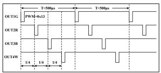
Figure 8 Phase Delay Mode 1 Timing
