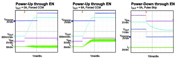
Power-Down through EN I<sub>OUT</sub> = 6A, Pulse Skip
