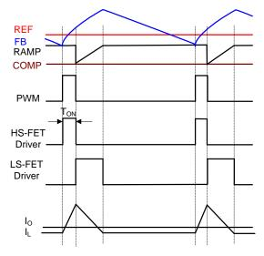
Figure 4: Pulse Skip in Light Load
