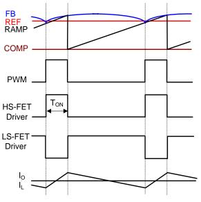
Figure 3: Heavy-Load Operation (PWM)
