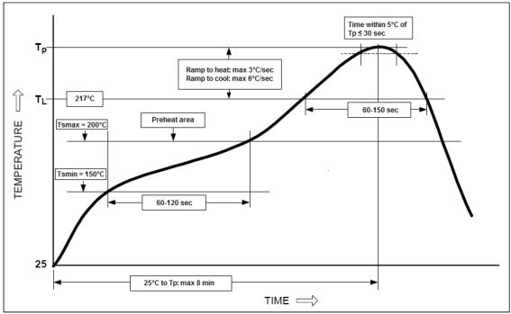
Figure 7: Reflow Temperature Profile
