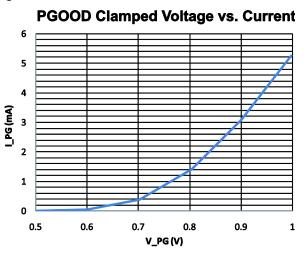
Figure 5: PGOOD Clamped Voltage vs. Pull-Up Current
