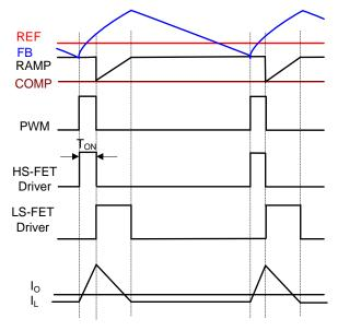
Figure 4: Pulse Skip in Light Load
