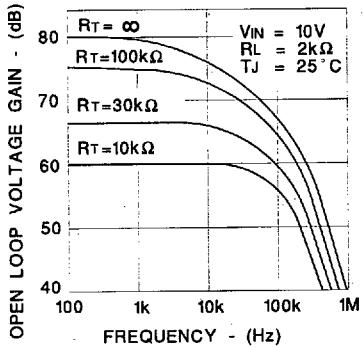
Note: R<sub>T</sub> is connected from Offset Pin to Gnd. Values of R<sub>T</sub> below 5.0k may cause Amplifier Cutoff at -55°C.
