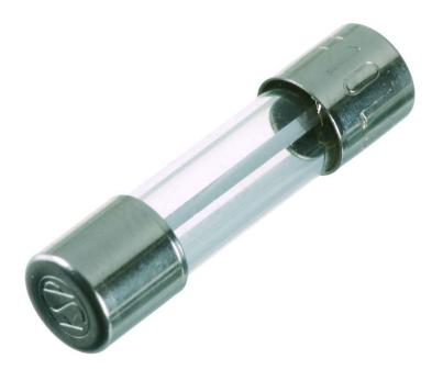
Fuse, Dimensions: 5x20 mm, Trigger characteristic: Fast-acting (F); Rated voltage: 250 V, Rated current: 8 A
