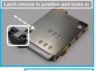
SIM Card is fully inserted
