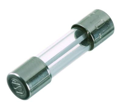
Fuse, Dimensions: 5x20 mm, Trigger characteristic: Fast-acting (F); Rated voltage: 250 V, Rated current: 2 A
