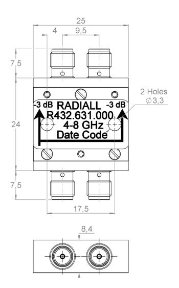
All dimensions are in mm. Tolerances according ISO 2768 m-H
