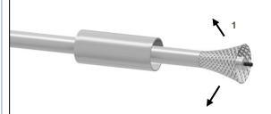
Push the connector body under the braid. Slide the ferrule over the braid.
