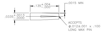
MATERIAL: BERYLLIUM COPPER PER ASTM B196, ALLOY C17300, TEMPER TD04.
