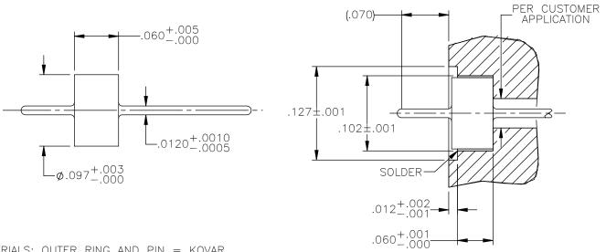
MATERIALS: OUTER RING AND PIN = KOVAR GLASS BEAD = CORNING 7070
