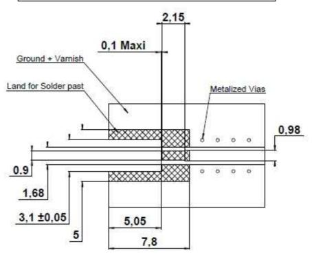
Dimensions applicable for Roger RO4350 PCB material thickness 0.508 mm , with ground layer on bottom . Applicable Frequency - DC to 12Ghz
