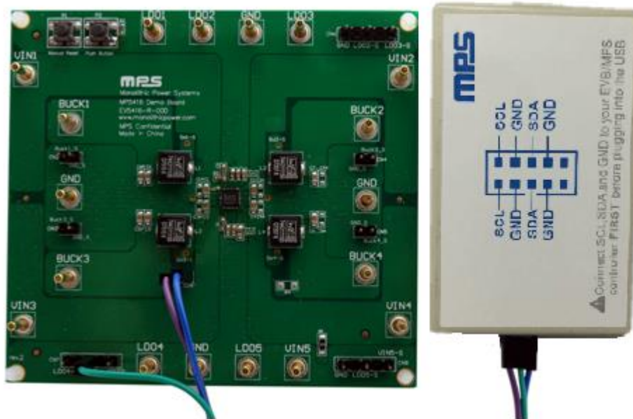
Figure 6: EVB to MPS I 2 C Communication Interface Device Wire Connection
