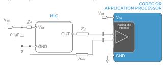
If necessary to improve RF performance, optional series components (resistors, ferrites, etc.) should be placed closest to the microphone pads. Bypass capacitors should be placed near each Vdd pin for best performance. Capacitors near the microphone should not contain Class 2 dielectrics due to their piezoelectric effect. Follow the codec manufacturer's recommendations for circuitry and layout.
