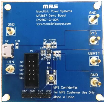
Figure 2: EV2667-G-00A Evaluation Board
