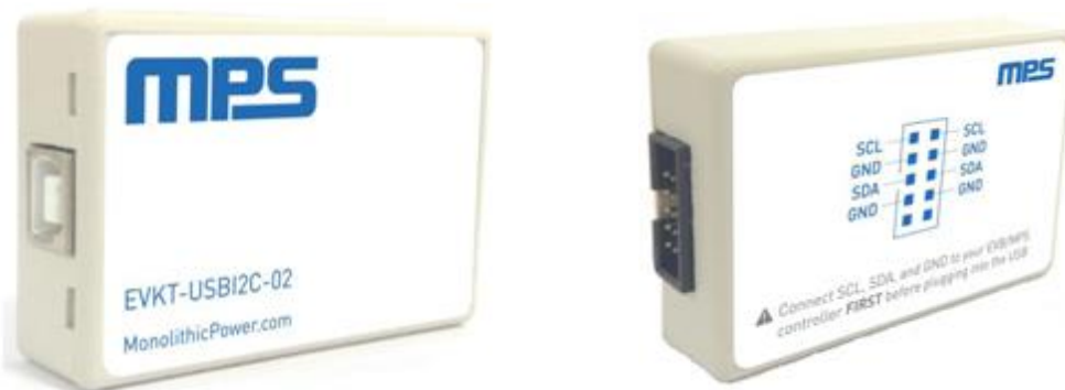
Figure 3: EVKT-USBI2C-02 Communication Interface
