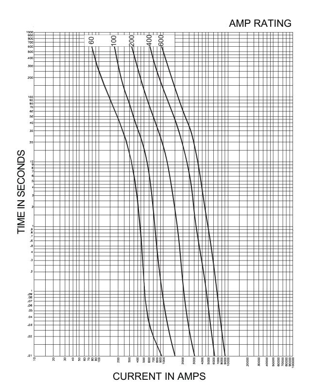
NOTE: 60 Amp fuse curve is ferrule style and included to show only relative performance. For actual 60 amp time-current curve performance, see data sheet no. 1003.
